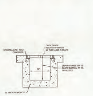
TRENCH DRAIN DETAIL NOT TO SCALE
